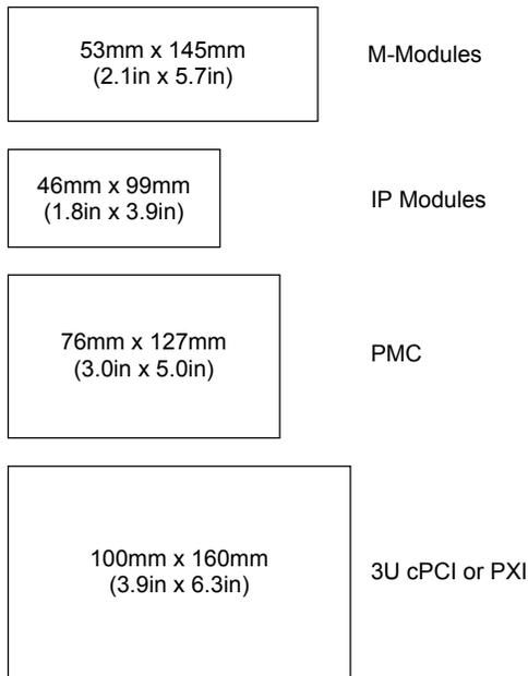
Figure 2. Relative size of various mezzanine modules
