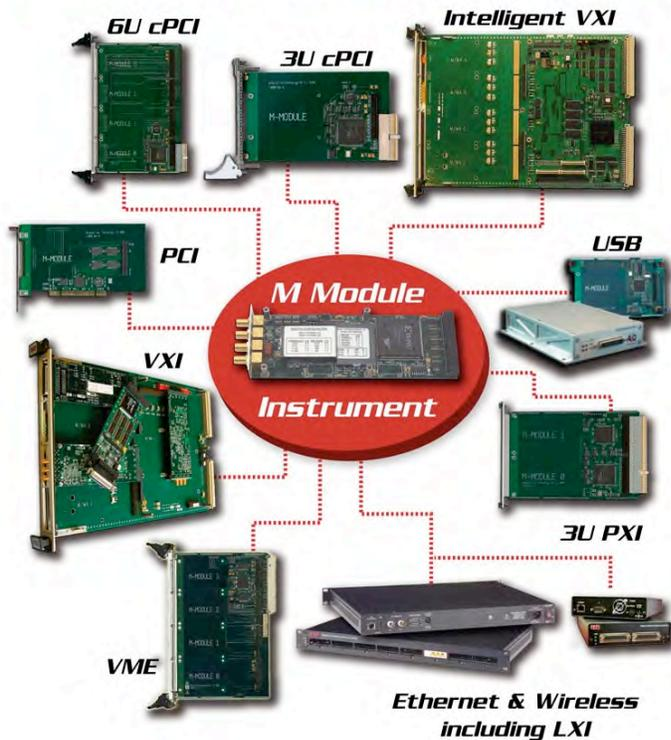
**Figure 4. Platforms where M-Module support is Available**
