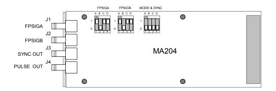
Figure 4. MA204 Hardware Configuration Switches
