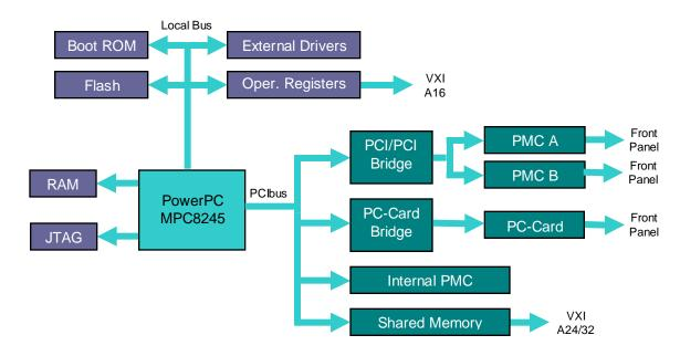
Figure 9 Device-Side Architecture
