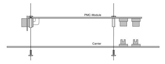
**Figure 1 PMC Module Installation**
