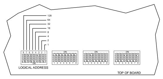
Figure 5 Logical Address Configuration Switch
