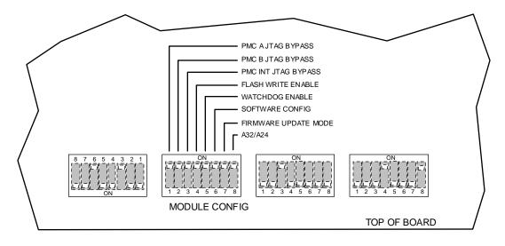
Figure 6 Module Configuration Switch
